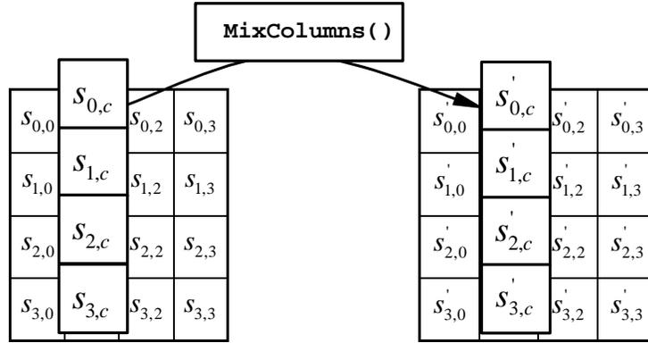
**Figure 9.** **MixColumns()** operates on the State column-by-column.
